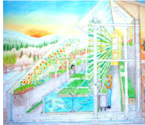
Schematic design of a passive-solar greenhouse from Anna Edey's influential book, Solviva (1998). Image: solviva.com
